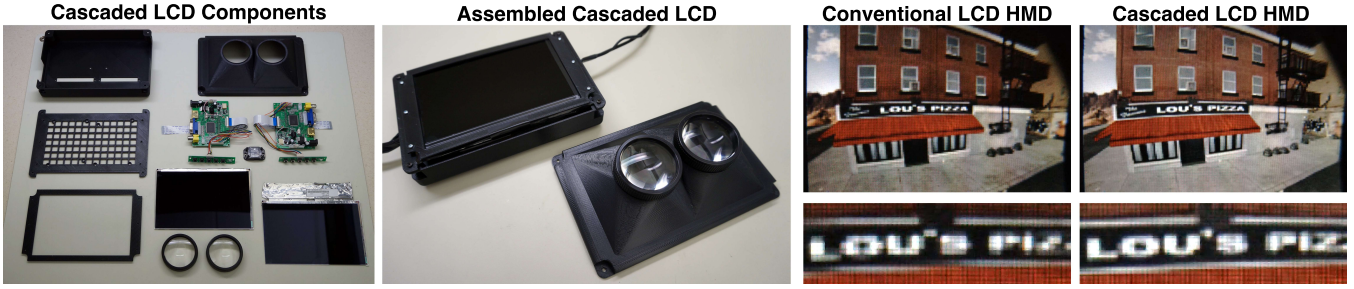
Figure 6: Cascaded LCD screen prototype. The custom-fabricated enclosure, interface electronics, IMU, magnifying optics, and modified panels are shown on the left. The assembled prototype supports both direct viewing and head-mounted display using the lens attachment. The two photographs on the right were taken through the magnifying optics to illustrate the HMD mode (using the real-time rank-1 factorization in Section 4.1). Note the improved legibility of text using the cascaded LCD, in comparison to a conventional (low-resolution) display.
