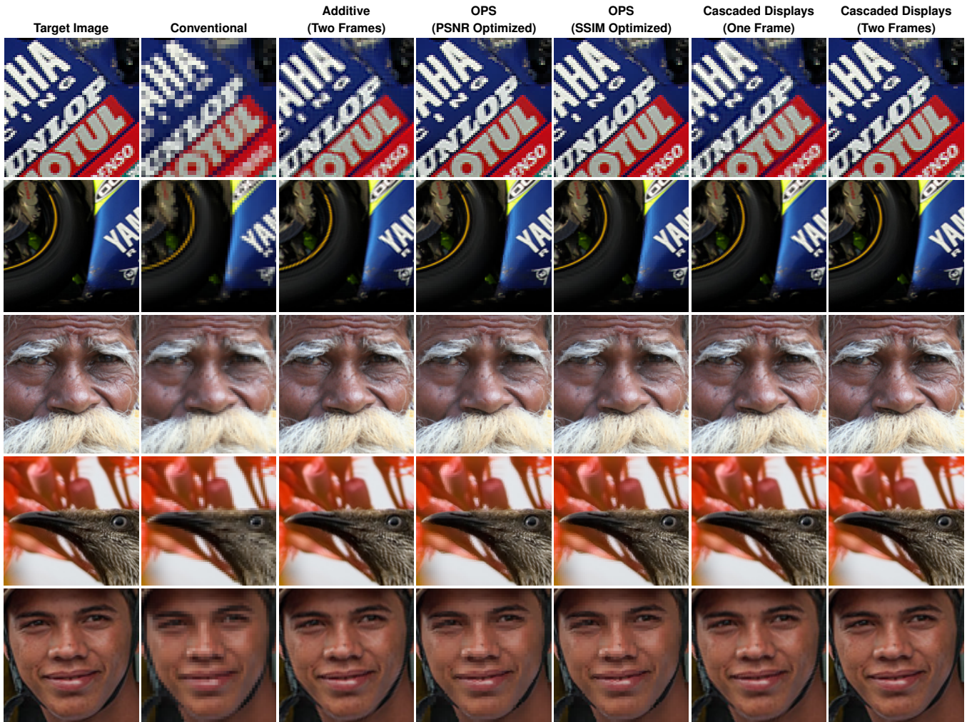
Figure 10: Visual comparison of superresolution displays. Image patches are reproduced with simulations of three different superresolution displays: additive superresolution using two frames, optical pixel sharing (OPS) using two frames with per-image PSNR- and SSIM-optimized edge thresholds and smoothing coefficients (see Section 5.2), and cascaded displays using one or two frames. Notice the enhancement relative to a conventional (low-resolution) display. Consult the supplementary data archive for the full set of comparisons. (Source images courtesy Yoshikazu Hara (first and second rows), Wen-Yan King (third row), JJ Harrison (fourth row), and Wilfredo R. Rodriguez H. (fifth row).)
